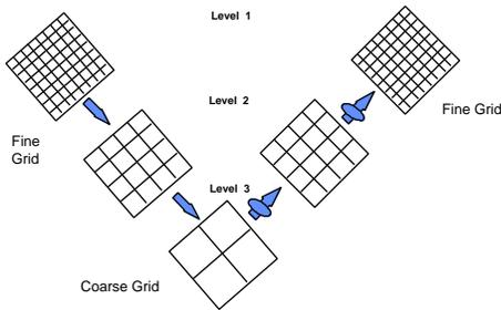
Fig 1 - Schematic showing the transfer of information from fine grid to coarse grid in the multigrid algorithm (Adapted from Bhogeswara and Killough, 1991)
