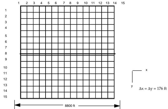
Fig 6 - Reservoir and Grid System of Test Problem 1 (Adapted from Data of Chang et al., 1992)
