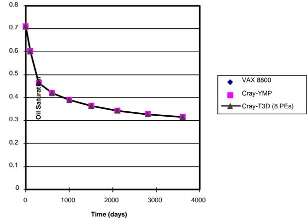
Fig 8 - Oil saturation - Time Profile for Test Problem 2
