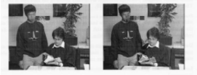
**Figure 3: Meaningless of the PSNR.** Left image: PSNR = 25.3dB, compression ratio = 12. Right image: PSNR = 27dB, compression ratio = 2. The left image has an higher visual quality for a better compression ratio although the PSNR is better for the right image.
