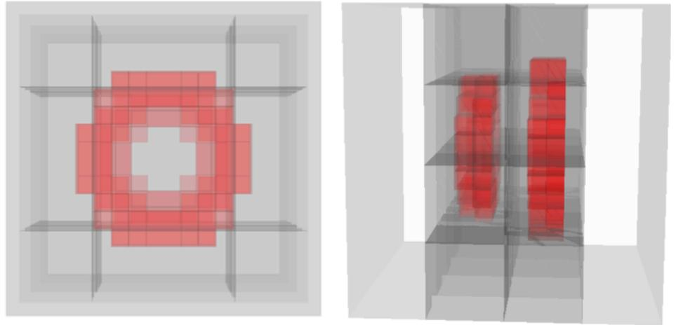
2 views (front and side) of one unit of AMR grid used in experiments. Grid has 3 levels. Refinement factor between levels is 4 (in each direction).
