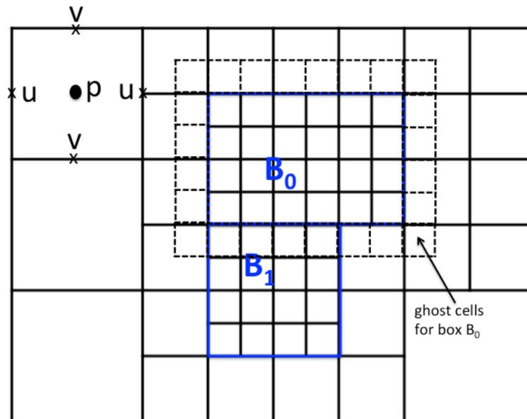
3 level AMR grid with 3 variables ( $u$ ,  $v$ ,  $p$ ). The refinement ratio is 2 in each direction
