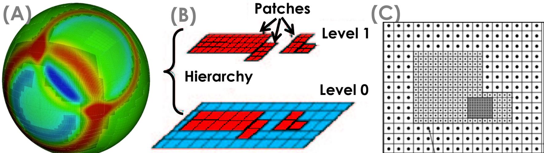
(A) An example of a space-time adaptive mesh refinement calculation in a cubed sphere geometry, for Climate applications. (B) The **hierarchical levels of mesh refinement** are used to capture moving features (e.g., multiple overlapping pressure waves). (C) Each **level of refinement** consists of a **group of patches**, each contains multiple data points, and each point belongs to a single patch. Tracked features can span patches or multiple levels as they evolve in time.
